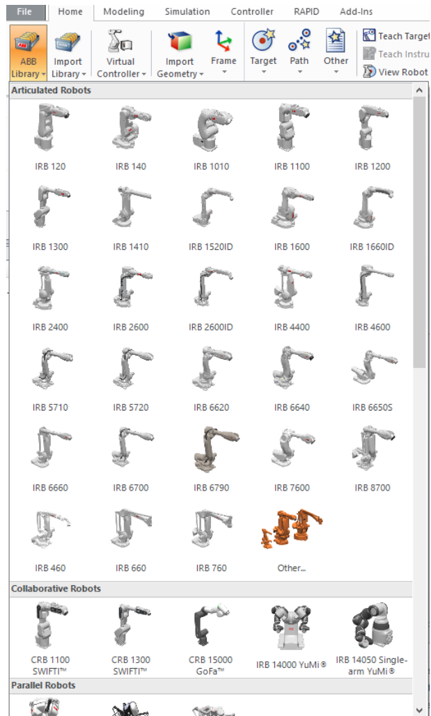
Slika 2.2.1.2 RobotStudio – izbornik Home – ABB Library
